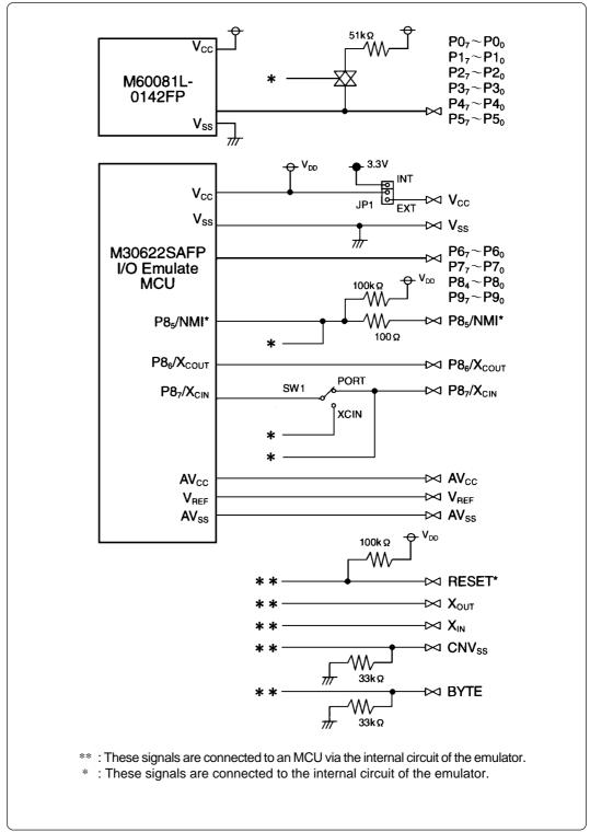
Figure 4.2 Connection diagram (emulation circuits)
